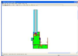
Modeling of windows, doors, skylights, walls, roofs, foundations, and other building envelope components is done for energy, moisture and structural performance. Several industry standard tools are used for this modeling, such as THERM, WINDOW, and WUFI and several in-house developed tools, such as FENSTRUCT and GLASTRUCT. Modeling is done for the purposes of determining performance of complex façade systems or for certification purposes, such as NFRC.
