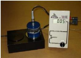
Thermal emissivity measurements are done for building materials using ASTM C1371 standard. Material samples with the minimum of 1 x 1 in., square or round (no upper limit in size) are measured using Devices and Services D&S Model AE1 portable emissometer. Wide range of emissivities can be measured with this instrument ranging from near mirror surfaces to near black bodies in Far Infra Red (FIR) wavelength range (normally from 2.5 µm to 50 µm).
